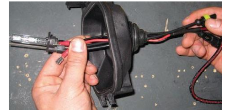
Feed wires through as shown above.
