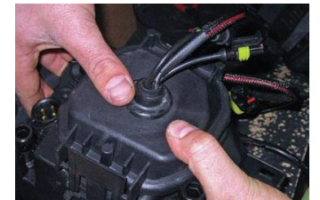
Make sure dust cap fits snug and wires are not being pulled.
